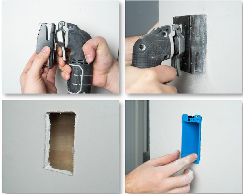
The Jonard Tools EBC-400 Electrical Wall Box Cutter is designed for cutting single gang boxes in drywall for installing old work boxes. The electrical wall box cutter features the following:
